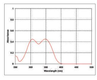
Tinuvin 571 exhibits strong absorbance in the 300-400 nm region and minimal absorbance in the visible region (>400 nm) of the spectrum. The absorption maxima are at 303 nm and 343 nm ( $\varepsilon = 14'210$  l/  $mol \cdot cm$ ) in chloroform solution.
